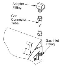
Figure 7 - Connecting Adapter to Gas Supply
